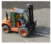
Forklifts typically run on LPG. Battery forklifts based on lead acid are in use but have challenges – they only run 6-8 hrs before needing a 16 hr recharge cycle, requiring removal of battery and special rooms for recharging.
